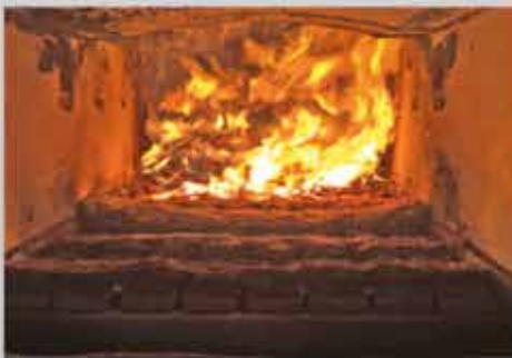
Pre-cast fire brick lined combustion chamber with moving step grate
