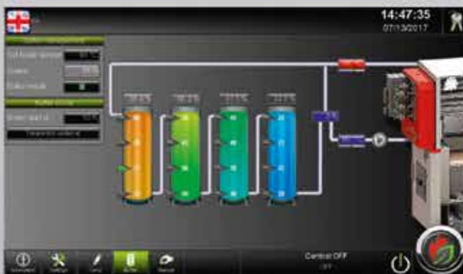
Buffer management for up to 4 buffer vessels with up to 4 temp. sensors each
