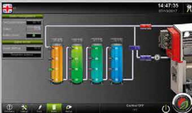
Buffer management for up to 4 buffer vessels with up to 4 temp. sensors each
