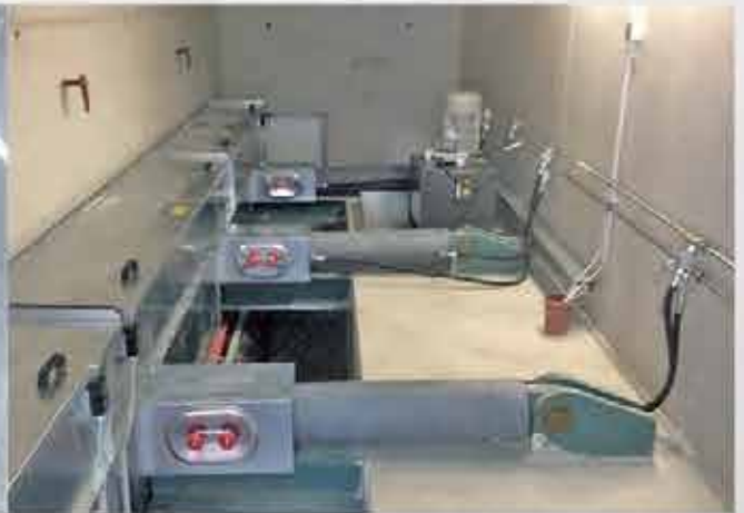
Robust hydraulic cylinder for walking floor movement
